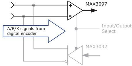
**CURRENT or VELOCITY COMMAND INPUTS: DIFFERENTIAL**
