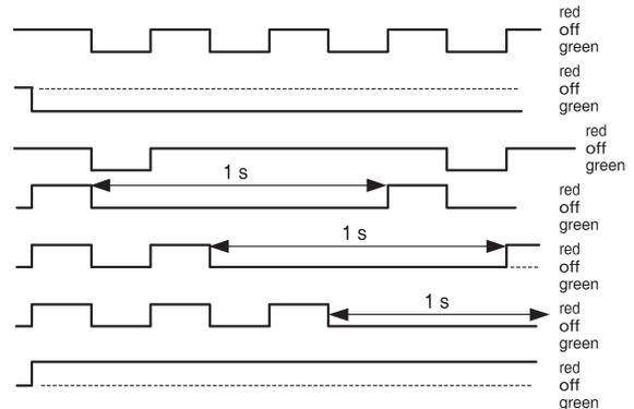
Note: Red & green led on-times do not overlap. LED color may be red, green, off, or flashing of either color.
