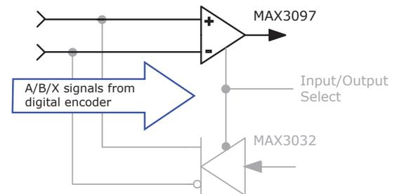
**AS DIGITAL COMMAND INPUTS IN PULSE/DIRECTION, PULSE-UP/PULSE-DOWN, OR DIGITAL QUADRATURE ENCODER FORMAT**
