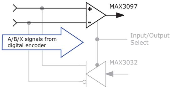
AS AN OUTPUT FOR FEEDBACK SIGNALS TO AN EXTERNAL CONTROLLER
