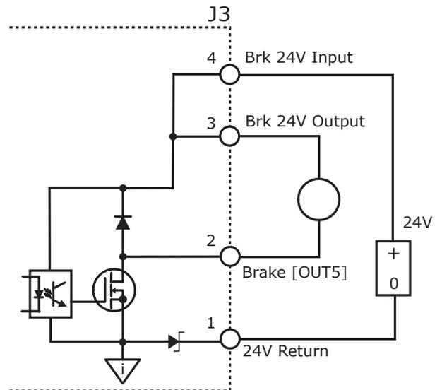
The brake circuits are optically isolated from all drive circuits and frame ground.
