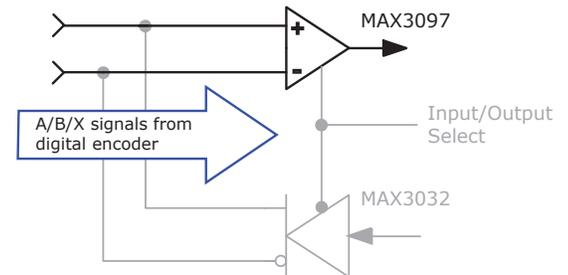
AS DIGITAL COMMAND INPUTS IN PULSE/DIRECTION, PULSE-UP/PULSE-DOWN, OR DIGITAL QUADRATURE ENCODER FORMAT
