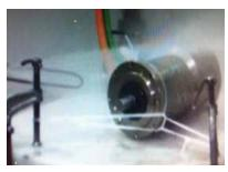
MPW motors were subjected to water intrusion tests as specified in DIN 40 050 part 9, section 7.4 at a level of protection of IP69K. Post-test inspection of the test units found no evidence of internal or external damage from water. Details of this test can be found on the MPW product page on parkermotion.com.
