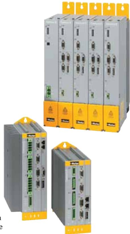
Although the Compax3 T30 uses standard resolver feedback, it can also be equipped with quadrature encoder, high-resolution Stegmann or SinCos® Hiperface™ encoder with single- or multi-turn absolute feedback capability or Heidenhain Endat 2.1.
